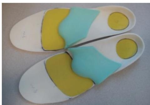
Custom foot orthoses during construction stage showing variable densities of material.
